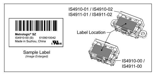
Figure 6. Serial Number Label Sample
